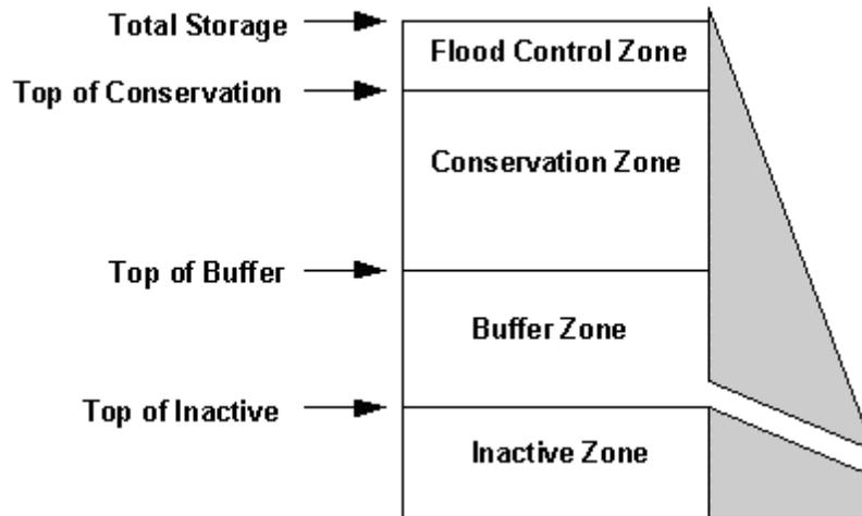
All of the water in the flood control and conservation zones is available for release, and equals the amount above Top Of Buffer (TOB and other reservoir zones levels are entered as data—see Supply and Resources\River\Reservoir\Operation),
