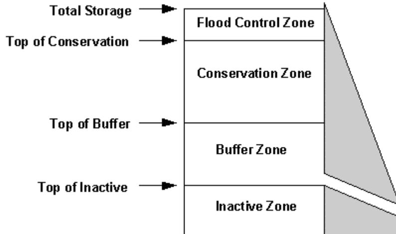
WEAP allows the reservoir to freely release water from the conservation pool to fully meet withdrawal and other downstream requirements. Once the storage level drops into the buffer pool, the release will be restricted according to the buffer coefficient, to conserve the reservoir's dwindling supplies. Water in the inactive pool is not available for allocation, although under extreme conditions evaporation may draw the reservoir into the inactive pool.
