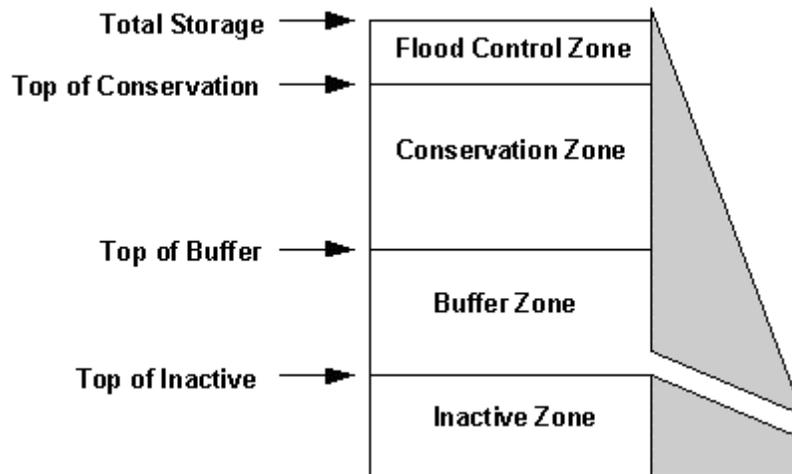
All of the water in the flood control and conservation zones is available for release, and equals the amount above Top Of Buffer (TOB and other reservoir zones levels are entered as data—see Supply and Resources\Local\Reservoir\Operation),
